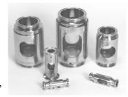
Other premium standard features include the use of borosilicate glass, a product contact surface of 0.6  $\mu m$  and an armored housing to help protect the glass from external objects and pipe stress. Units can be used during SIP/CIP and sterilizing/autoclaving. Units are available in tube OD sizes from 3/8 to 4 inches as standard (Smaller or bigger sizes are also available on request) and ratings
